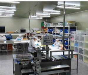
Clean room ISO 14644-1 Class 8 or 100,000 : 0.5µm/ft 3
